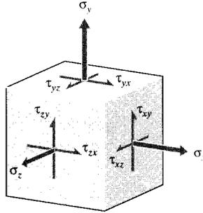
Figure 4: Cartesian Cauchy stress components in three dimensions.
