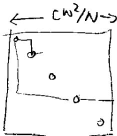
By adjusting  $c$ , can route edges within mesh + room on perimeter for wires to escape.
