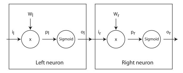
Note that the subscripts indicate layer. Thus,  $i_l$ ,  $w_l$ ,  $p_l$ , and  $o_l$  are the input, weight, product, and output associated with the neuron on the left while  $i_r$ ,  $w_r$ ,  $p_r$ , and  $o_r$  are the input, weight, product, and output associated with the neuron on the right. Of course,  $o_l = i_r$ .
