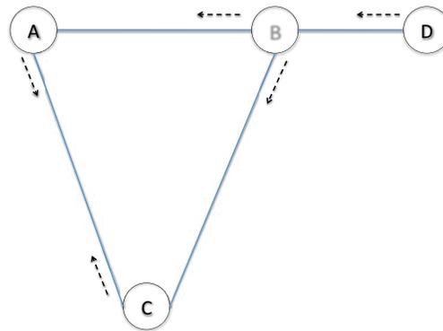
Figure 18-2: Split horizon (with or without poison reverse) doesn't prevent routing loops of three or more hops. The dashed arrows show the routing advertisements for destination  $D$ . If link  $BD$  fails, as explained in the text, it is possible for a "count-to-infinity" routing loop involving  $A$ ,  $B$ , and  $C$  to ensue.
