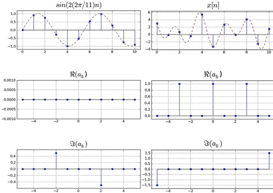
Figure 13-2: The spectrum of two periodic signals, plotted as a function of the frequency index,  $k$ , showing the real and imaginary parts for each case.  $P = 11$  (odd).
