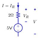
Voltage across resistor:  $V_R = V - 5$ .
