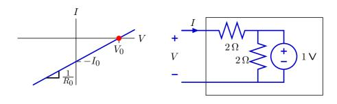
Set I=0 in the circuit. Then  $V=V_0=1$ V.
