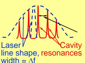
$$\begin{split} \frac{m\lambda_m}{2} &= L \quad (\text{mirrors } \approx \text{ short circuits}) \\ \lambda_m &= \frac{2L}{m}, \ f_m = \frac{cm}{2LN} \quad (\text{N} = \text{refractive index}) \\ f_{i+1} - f_i &= \frac{c}{2LN} \end{split}$$
