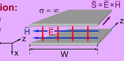
Currents in Plates:  $\oint_C \overline{H} \bullet d\overline{s} = \iint_A \overline{J} \bullet d\overline{a} = I(z)$  I(z) = H(z)W, independent of path C Surface Currents  $J_s(A m^{-1})$ :  $\overline{J}_s(z) = \hat{n} \times \overline{H}(z)$  [A m<sup>-1</sup>]
