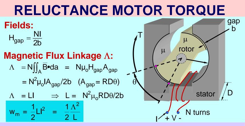
Set V = dA/dt = 0:  $T = -\frac{dw_{m}}{d\theta} = -\frac{\Lambda^{2}}{2}\frac{dL^{-1}}{d\theta} = \frac{\Lambda^{2}}{2}\frac{2b}{N^{2}\mu_{o}RD\theta^{2}} \quad [\propto l^{2}], \Lambda = N\mu_{o}H_{gap}R\theta D$   $= \frac{1}{2}\mu_{o}H_{gap}^{2}2bDR = \frac{W_{gap}}{d\theta}\frac{dV_{olume}}{d\theta} \quad [Nm] \text{ Torque}$ We power coil until overlap is maximum, then coast until it is zero Magnetic pressure = Energy density [J/m^{3} = N/m^{2}]
