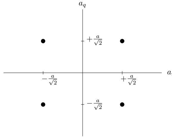
FIGURE 12.9  $I$ - $Q$  Constellation for quadrature phase-shift-keying (QPSK).
