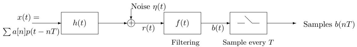
FIGURE 12.2 Transmitter, channel and receiver model for a PAM system.
