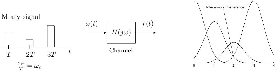
FIGURE 12.3 Illustration of Inter-symbol Interference (ISI).
