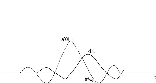
FIGURE 12.4 Illustration of the no-ISI property for PAM when  $g(0) = 1$  and  $g(t) = 0$  at other integer multiples of the inter-symbol time  $T$ .
