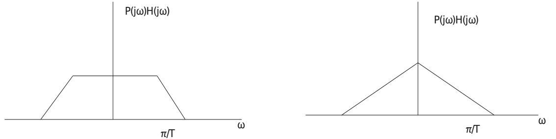
FIGURE 12.5 Two possible choices for the Fourier transform of pulses that decay in time as  $1/t^2$  and satisfy the Nyquist zero-ISI condition for appropriate choice of  $T$ .
