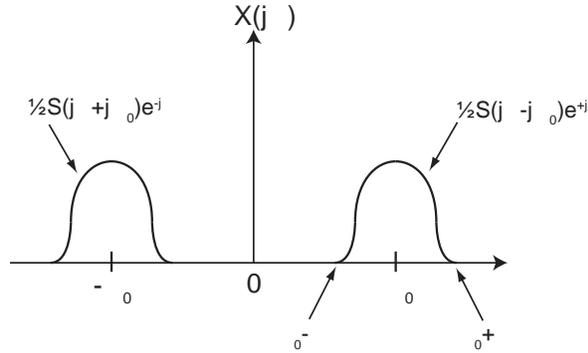
FIGURE 3.2 Spectrum of  $x(t)$  with  $s(t)$  narrowband
