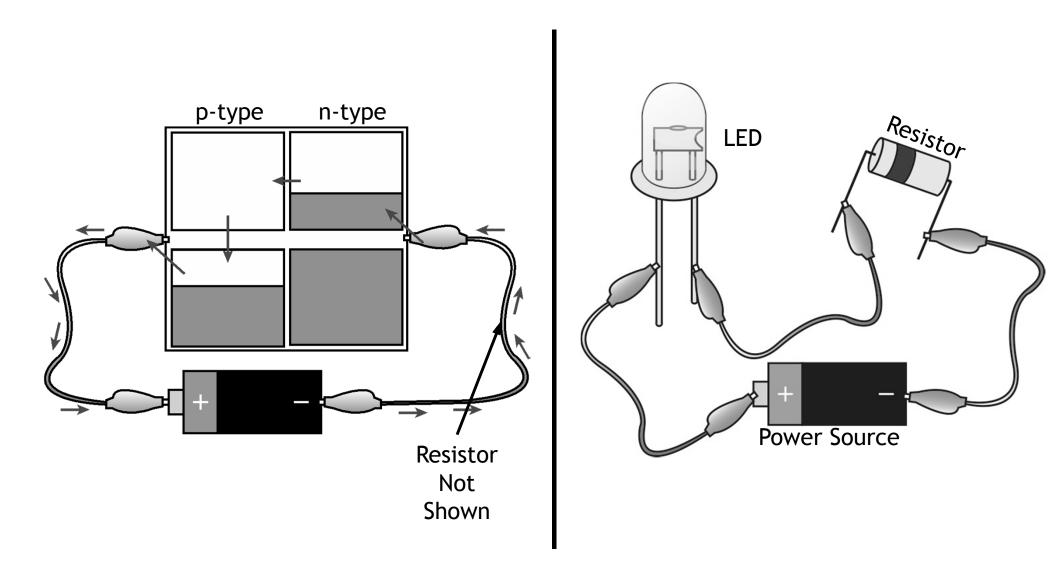
High energy electrons (n-type) fall into low energy holes (p-type)
