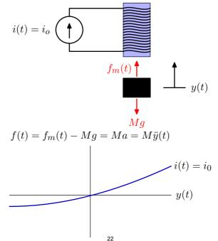
Represent the magnet as a system: input y(t) and output f(t).
