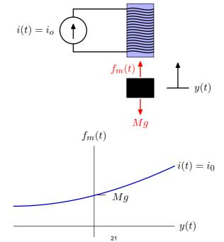
The net force  $f(t) = f_m(t) - Mg$  accelerates the mass.
