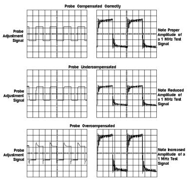
Figure 4 Oscilloscope Probe Compensation
