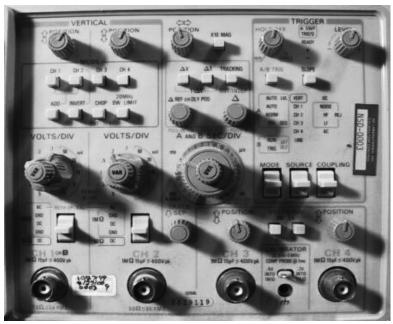
Figure 3 Control Panel for the Tektronix 2445 Oscilloscope
