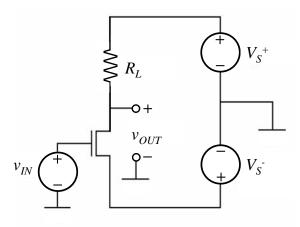
Figure 1: Amplifier Dual power supplies layout.
