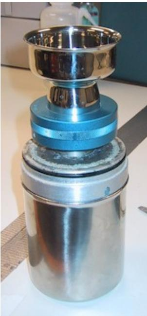
Figure 2: Millipore Field Apparatus
