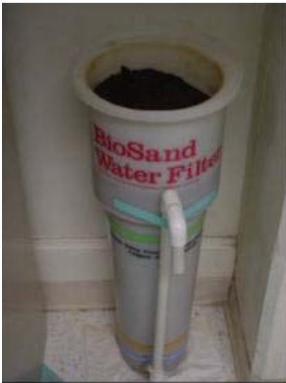
Figure 7. A prototype combined-filter
