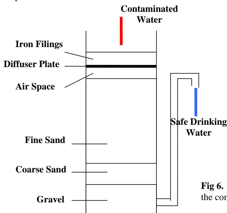
**Fig 6.** A schematic diagram of the combined-filter
