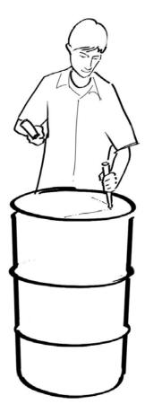
Cut a large opening for filling the kiln with the material you want to carbonize. Cut several holes in the bottom of the drum. These holes allow air to flow through the drum while burning, which results in a hotter fire and produces better charcoal.
