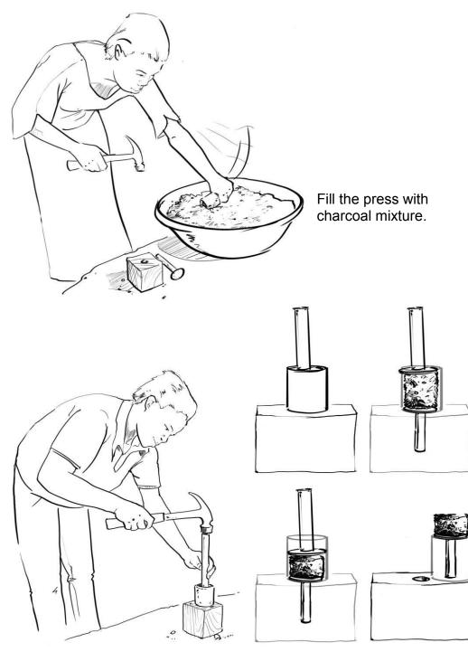
Hit plunger to form the briquette. ejector to remove the briquette.
