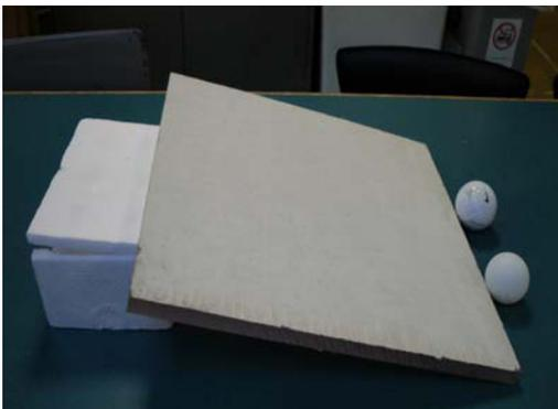
I have set up an experiment to study the rolling motion of different types of objects down to the plane. The objects included a solid sphere ball, a spherical shell, a solid cylinder and a cylindrical shell. All objects have approximately equal diameter. The setting up and the procedures are written on my journal which I will scan and attach to another submission for reference. The distance traveled by all objects are the same.
