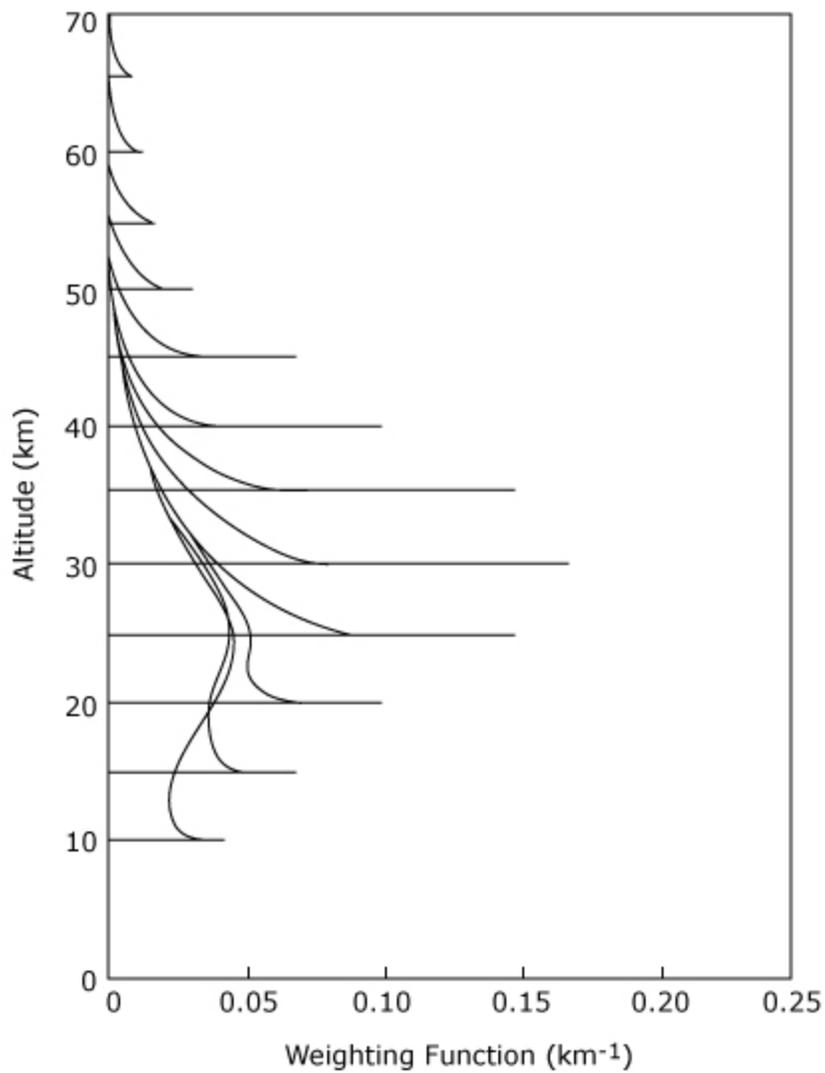
Limb viewing weighting function for the ideal case of an instrument with an infinitesimal vertical field of view for the spectral band 585-705  $\text{cm}^{-1}$  covering most of the 15  $\mu\text{m}$  band of  $\text{CO}_2$ .
