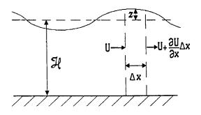
Figure 11.1: Shallow water geometry.
