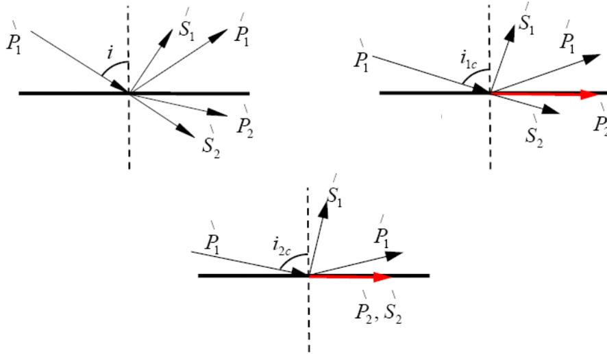
Since, P-SV are coupled, we need a SV wave to satisfy the boundary conditions. Let incident P wave make an angle 'i', transmitted P wave - angle 'j' and transmitted SV wave –angle 'k' with the normal respectively.
