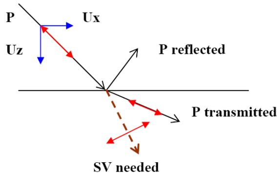
**NOTE:** In general, P-SV and SH waves are not decoupled. They are only if the medium is isotropic (heterogeneity is permissible) and if the normal at an interface is in the plane of propagation.
