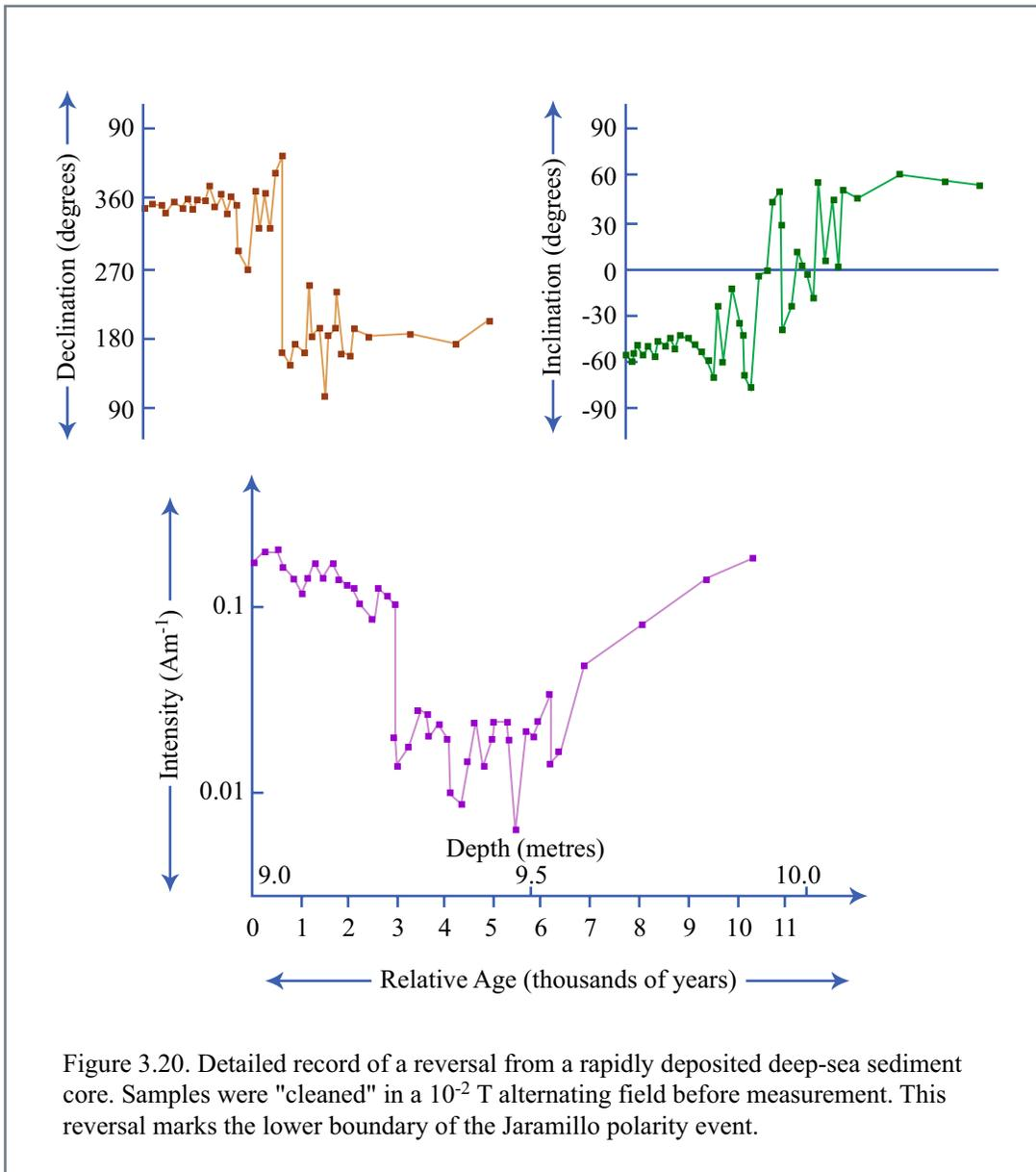
Figure 3.20. Detailed record of a reversal from a rapidly deposited deep-sea sediment core. Samples were "cleaned" in a  $10^{-2}$  T alternating field before measurement. This reversal marks the lower boundary of the Jaromillo polarity event.
