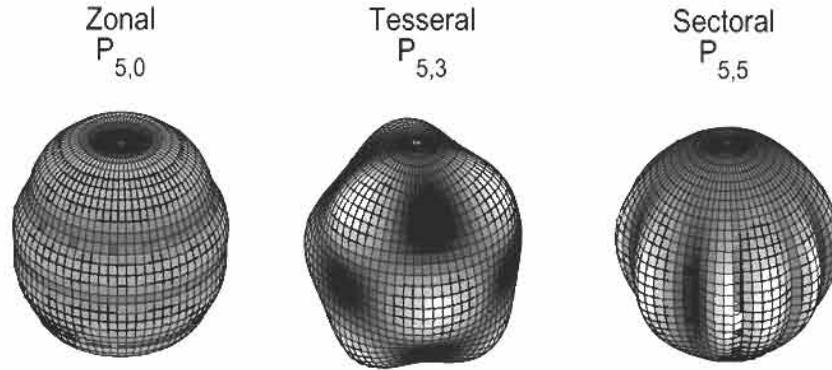
Figure 2.15: Zonal, tesseral and sectoral spherical harmonics.
