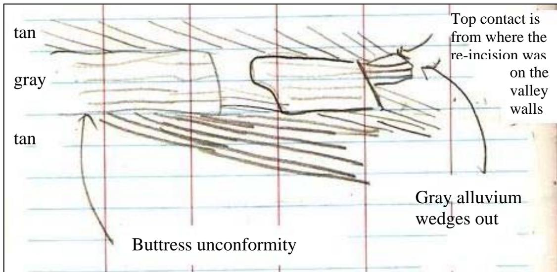
Figure 58: Sketch of buttress unconformity between the older tan and newer gray alluvium in Afton Canyon
