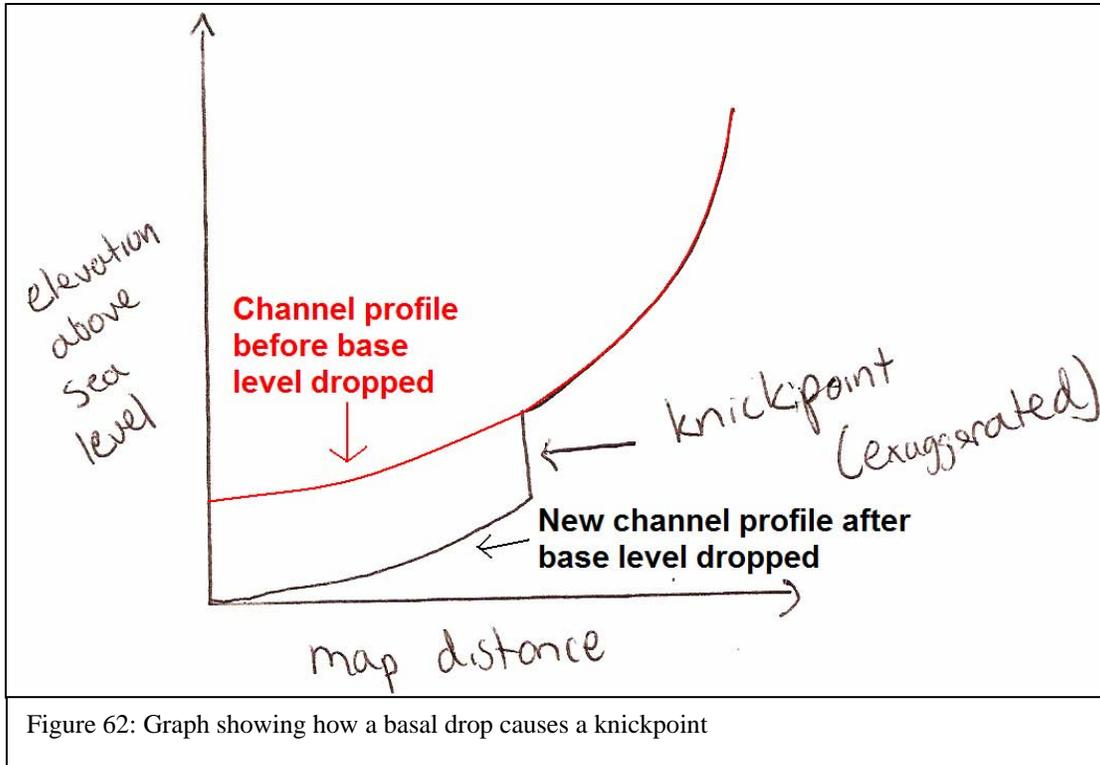
Figure 62: Graph showing how a basal drop causes a knickpoint
