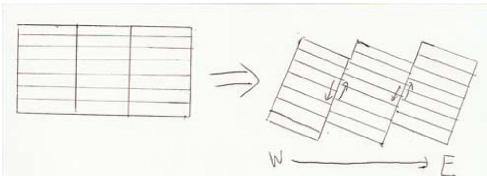
Figure 36: Diagram of classic block faulting which results in beds dipping to the east, as seen in the southern end of the Nopah Range
