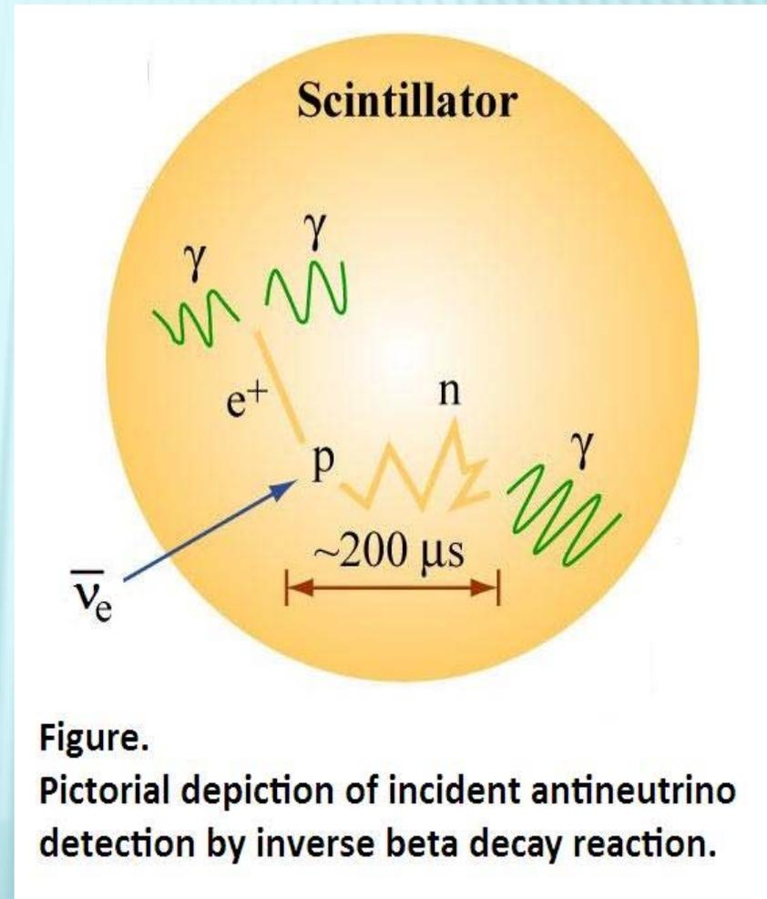
Figure. Pictorial depiction of incident antineutrino detection by inverse beta decay reaction.
