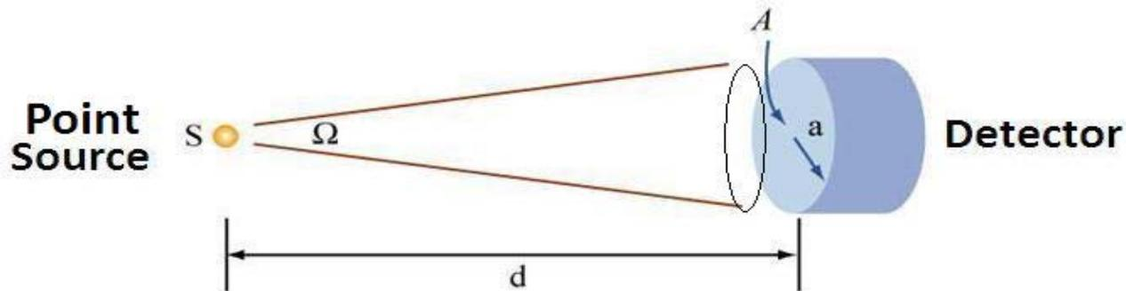
Figure. Pictorial depiction of solid angle subtended between source and detector.
