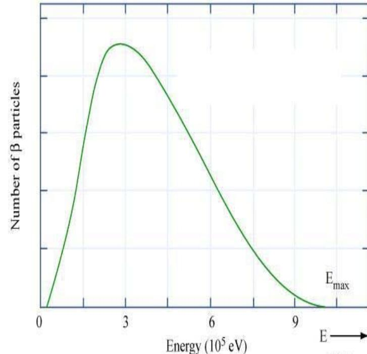
Figure. Energy Spectrum of the  $\beta$  rays from  $^{210}\text{Bi}$
